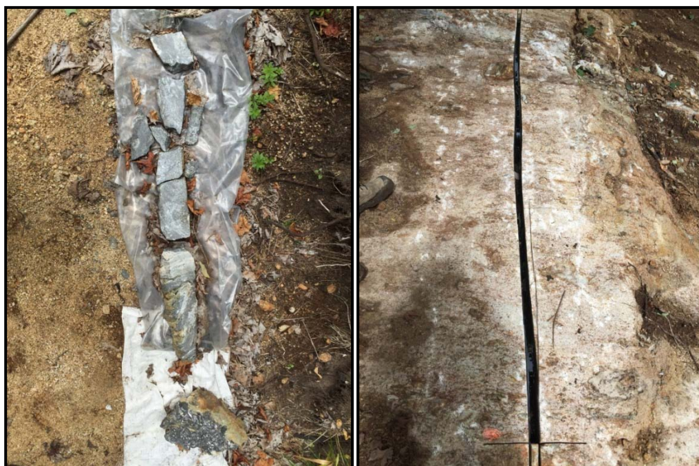
Figure 10-4: Example of Channel Sample Witness (left) and Channel (right)
